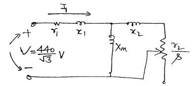
where  $r_1 = 0.294 \ \Omega$ ;  $x_1 = 0.503 \ \Omega$ ;  $X_m = 13.25 \ \Omega$ ;  $r_2 = 0.209 \ \Omega$ ;  $x_2 = 0.144 \ \Omega$ .
